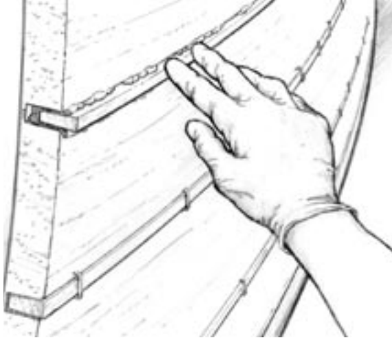
Figure 6-4 Push the wet-out spline into the seam.
