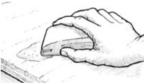
Figure 3-14 Sand the fairing compound to the desired shape after the epoxy has reached final cure.
