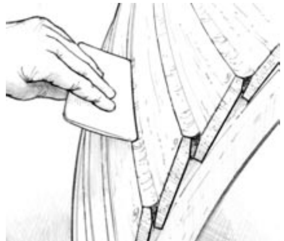
Figure 6-9 Fill the wet-out seam with thickened epoxy.
