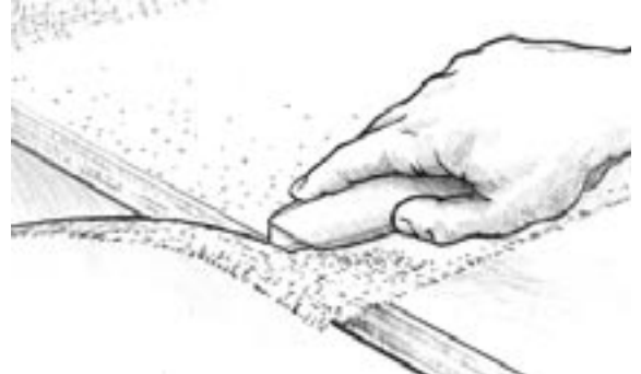
Figure 3-16 Trim excess cloth when the epoxy reaches initial cure. The wet-out cloth will be dry but still flexible, and will trim easily with a sharp utility knife.
