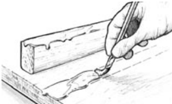
Figure 3-6 Wet out the bonding surface with unthickened epoxy for maximum penetration and to prevent resin-starved joints.
