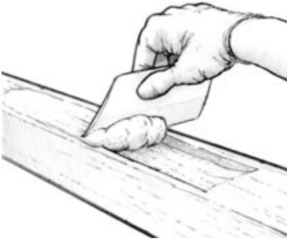
Figure 4-2 Trowel thickened epoxy into smaller voids.
