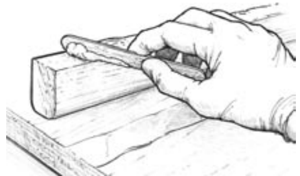
Figure 3-7 Apply enough thickened epoxy to one of the bonding surfaces to squeeze out of the joint slightly when clamped.
