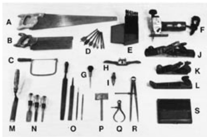
Figure 2 – Broader tool inventory: (A) crosscut saw; (B) back saw; (C) coping saw; (D) large set spade bits; (E) large set drill bits; (F) electric saber saw; (G) awl; (H) spokeshave; (I) plumb bob; (J) jack plane; (K) bench or smoothing plane; (L) Surform tool; (M) offset chisel; (N) chisel assortment; (O) file & rasp assortment; (P) protractor; (Q) calipers; (R) dividers; (S) whetstone.
