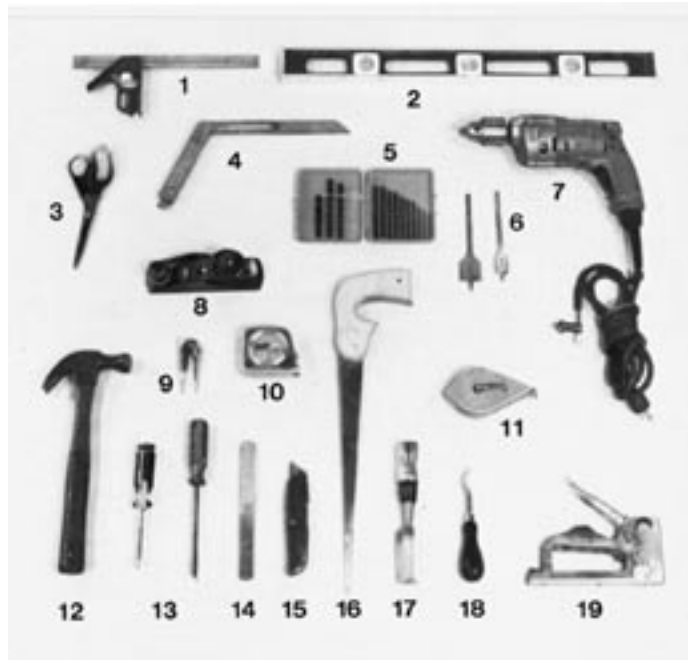
Figure 1 – Minimal tool inventory: (1) combination square; (2) 600mm level; (3) scissors; (4) sliding bevel or bevel square; (5) standard drill bits; (6) spade drill bits; (7) electric drill motor; (8) block plane; (9) compass; (10) 7,0 m measuring tape; (11) chalk line; (12) hammer; (13) screwdrivers; (14) rasp; (15) utility knife; (16) keyhole saw; (17) chisel; (18) staple removing tool; (19) staple gun.
