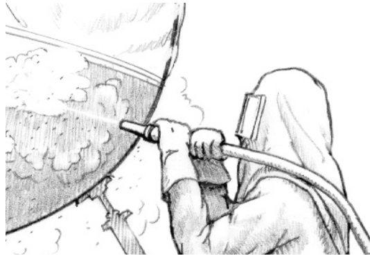
Figure 4.3. Sandblasting is a common method of opening blisters and abrading the hull
