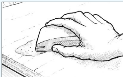
Figure 23 Sand cured fairing compound to desired contour.
