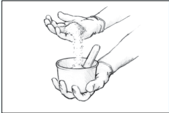
Figure 4 Stir in small quantities of filler until the desired consistency is reached.
