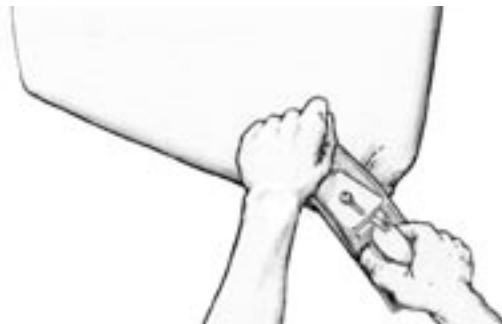
Figure 8-3 Plane or file the remainder of the bulge flush after you have forged as much as is practical.
