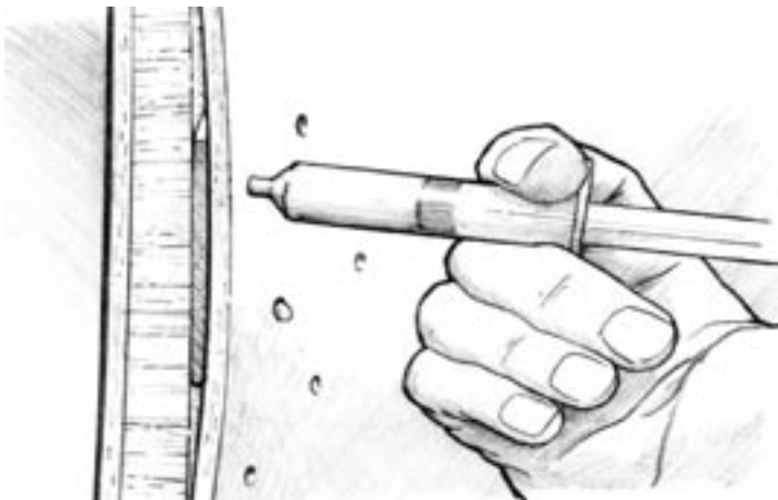
Figure 5-1 Inject epoxy under the skin using an 807 syringe with the tip cut off to match the hole diameter.
