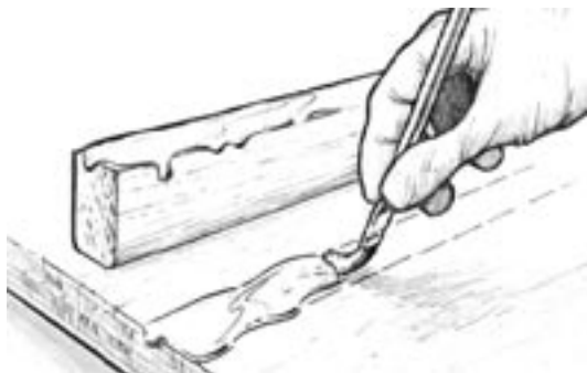
Figure 9-8 Wet out bonding surfaces with unthickened epoxy for maximum penetration and greater adhesion.
