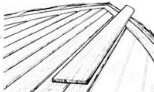
Figure 6-4 Cut and fit the teak strips. Mask off and protect surrounding surfaces.
