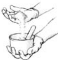
Figure 9-7 Blend in small handfuls or scoops of the appropriate filler until the desired consistency is reached.
