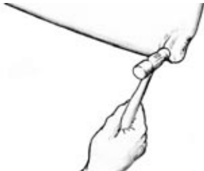
Figure 8-2 Use a ball peen hammer, with repeated light taps to work the lead bulge back to its original shape.
