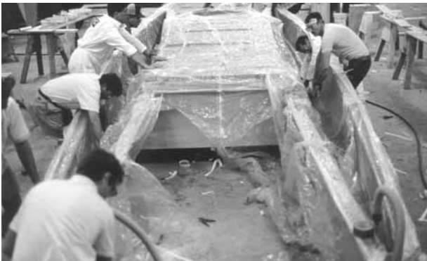
Figure 4-6 The laminate's position is checked as the vacuum is being applied. Note that there is plenty of extra bag to allow for the depth of the mold. Narrow bag material can be joined with mastic into larger sheets.
