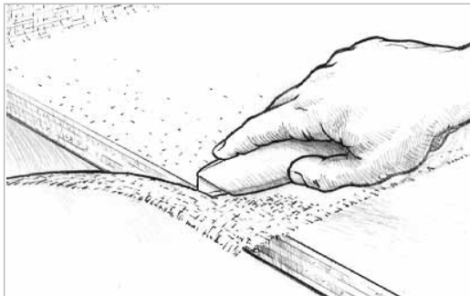
Figure 5-19 Trim excess cloth when the epoxy reaches its initial cure phase. The wet-out cloth will be dry but flexible and will trim easily with a sharp utility
