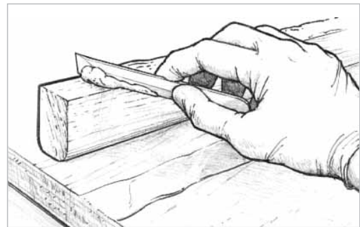
Figure 5-9 Apply enough thickened epoxy to one of the bonding surfaces so that a small amount will squeeze out of the joint when clamped with moderate pressure.
