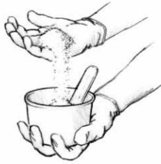
Figure A-5 Stir in small handfuls of filler until the desired consistency is reached.
