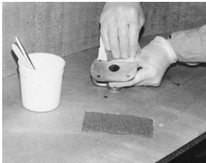
Figure 14-14 Wet sand the epoxy into the bonding surface.
