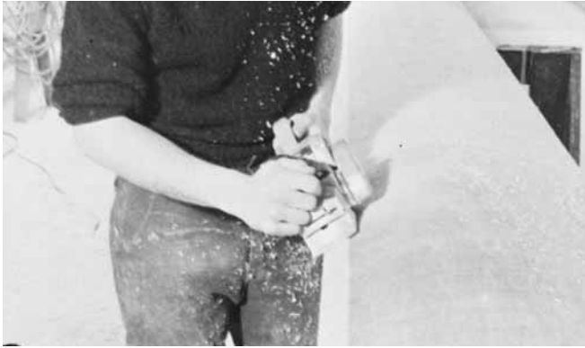
Figure 8-7 An electric plane used here to trim a wing mast during construction.
