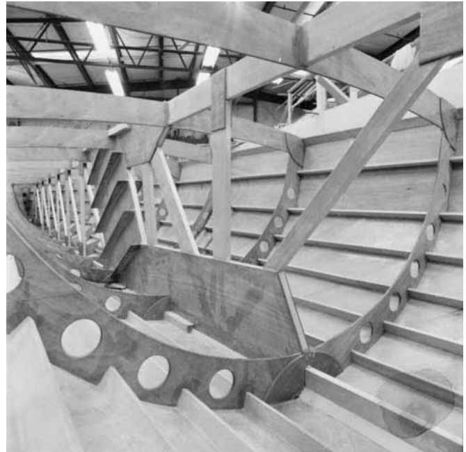
Figure 5-7 Looking forward in the main hull of the 60' (18.2m) proa Slingshot . The stringer-frame method is easily adapted to fairly sophisticated designs for boats of any size.
