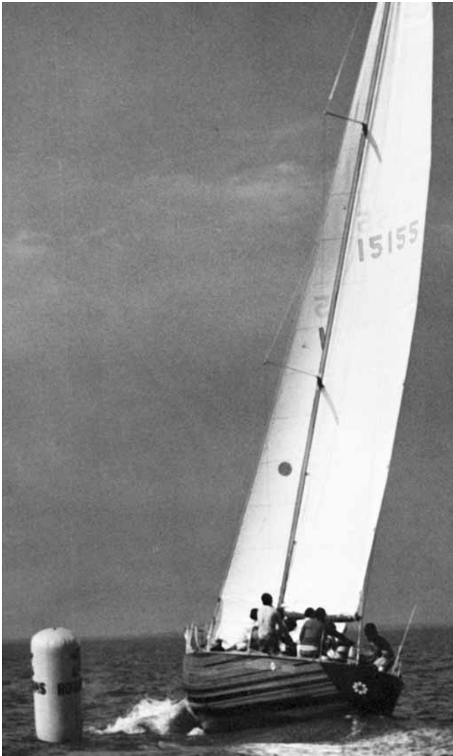
Figure 5-5 The 42' (12.8m), Ron Holland designed, IOR 2-ton racer Golden Dazy was built by Gougeon Brothers using the strip plank/veneer method.
