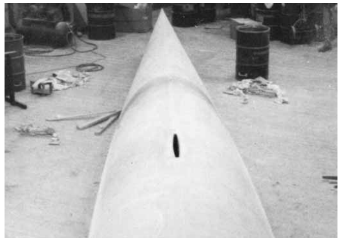
Figure 15-4 Bottom of the proa Slingshot has been coated with gray 420 Aluminum Powder pigmented epoxy and sanded in preparation for painting.
