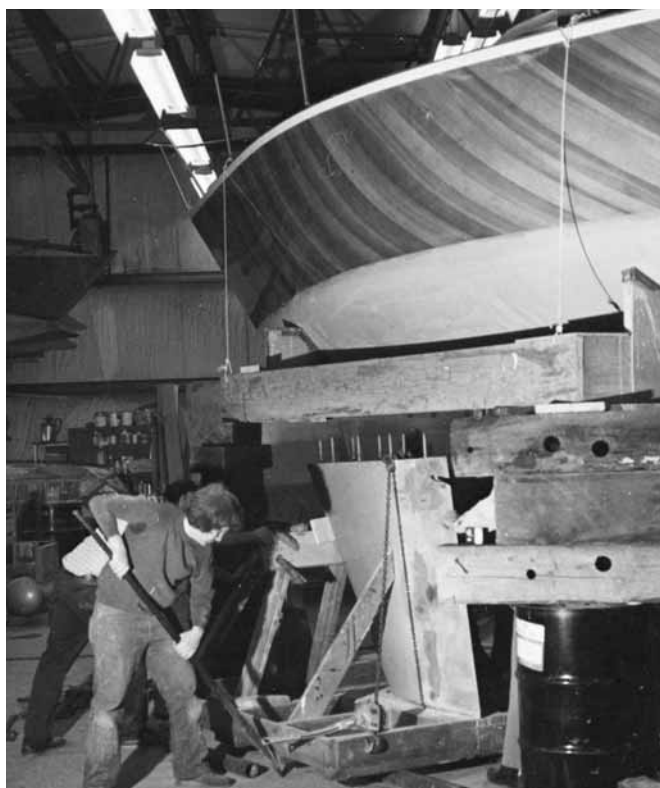
Figure 14-24 Rolling a 10,000-pound keel into position on a handling fixture. The keel can be shifted slightly from side to side and fore and aft.
