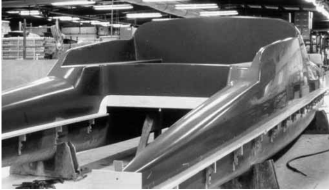
Figure 20-2 A plug for a 32' (9.7m) catamaran is polished and waxed, ready for a mold to be cast. The mold for the upper surface will be female in the areas of the hulls and cabin top and male in the cockpit area.
