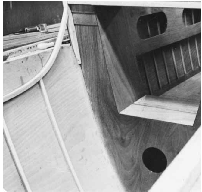
Figure 25-21 Laminated frames, a box-type bulkhead, and shelf and bunk bottoms all support the developed plywood skin on this 35' (10.6m) racing trimaran.
