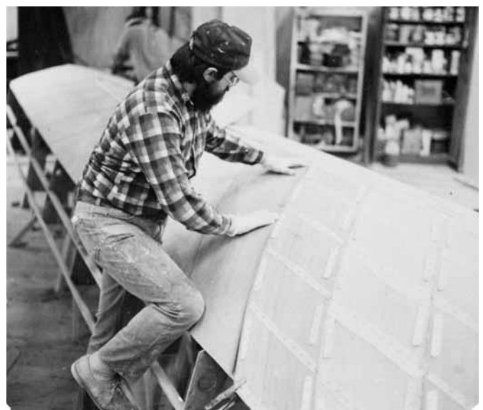
Figure 21-13 Fitting a veneer against a previously bonded plank.
