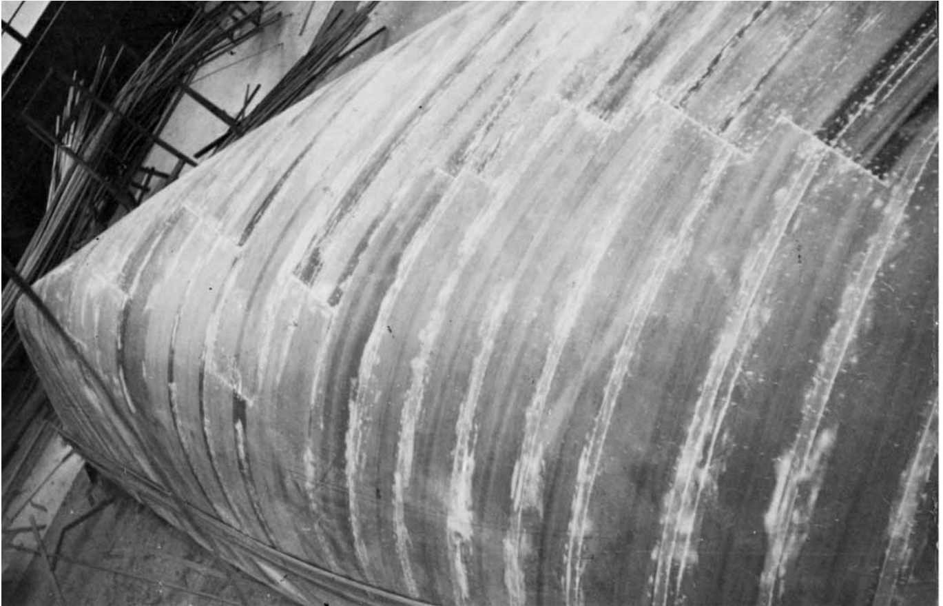
Figure 21-3 Veneers in interlaminated layers of this laminated hull are butted randomly. This reduces scrap and eases lay up without sacrificing the strength of the hull. Note the final layer of veneer being laid fore and aft at the lower left.
