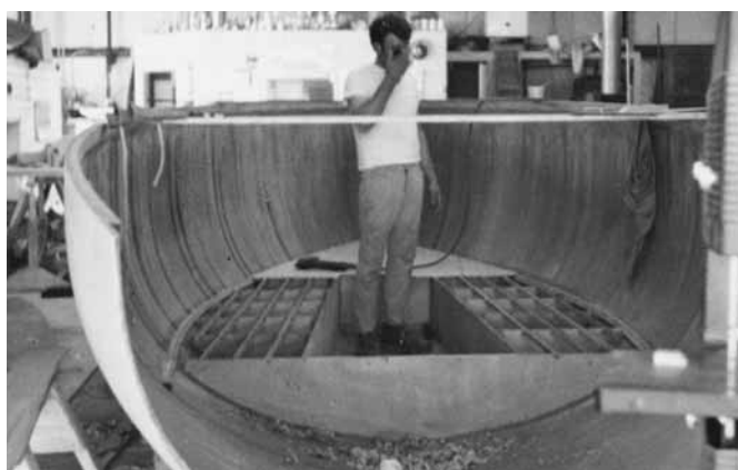
Figure 26-6 The transom is left open for easy access to the interior. Structural bunks are also airtight buoyancy tanks for this lightweight laminated sloop.
