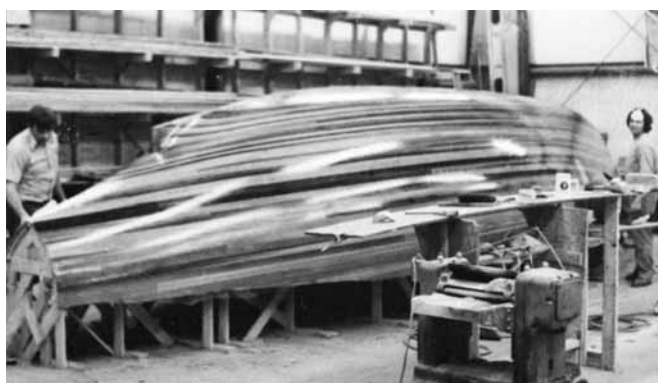
Figure 15-1 Coating the exterior of an IOR ½-ton racer. This boat has a natural finish. All fairing, finish sanding, and coating were done prior to removing the hull from the mold.
