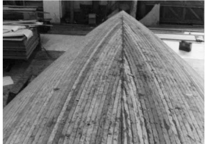
Figure 23-7 The keel joint of the 42' (12.8m) hull shown in Figure 23-4. Note the pattern of screw holes where the planks are secured to the mold frames.
