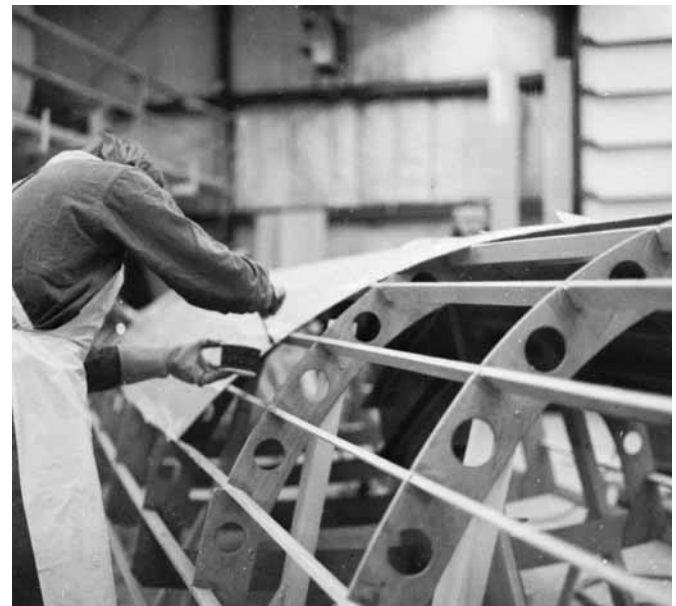
Figure 21-10 Applying epoxy to the edge of a previously fastened plank.
