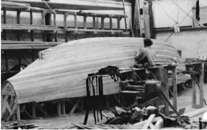
Figure 21-22 The final layer of veneer is laid fore and aft on this IOR ½-ton racer.
