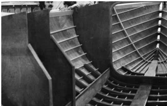
Figure 26-5 Interior of the IOR ½ ton after righting, before completion of interior details and installation of hardware and the engine.
