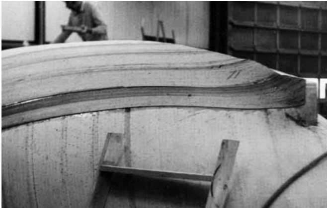
Figure 21-5 More staples are necessary to hold down thin veneers in a reverse or concave area near a skeg. Note the reasonably regular stapling patterns employed on planking in the foreground.
