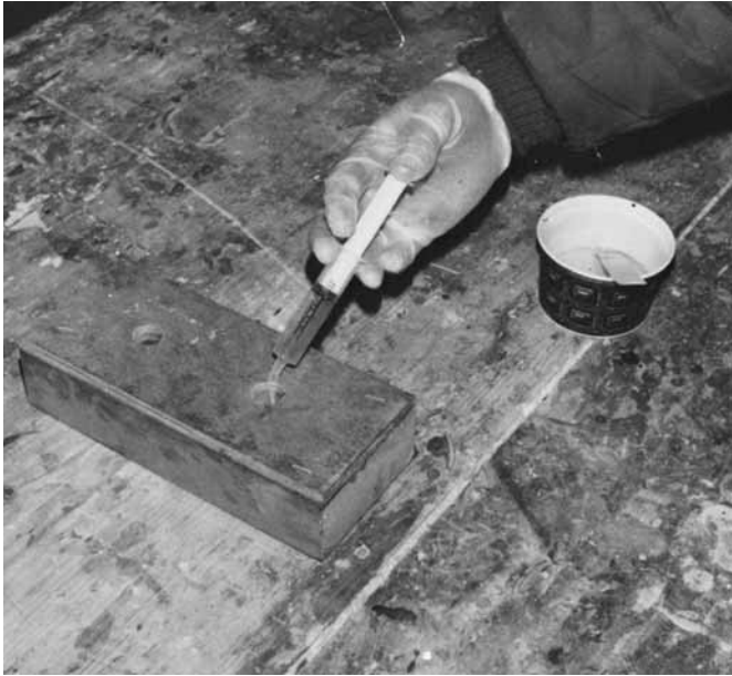
Figure 14-10 Use a syringe to fill oversized holes.
