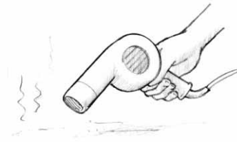
Figure A-7 Dry the surface. Allow wet surfaces to dry thoroughly or use heat or a fan to speed drying.
