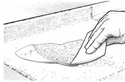
Figure A-24 Spread epoxy over the cloth surface with a plastic spreader.
