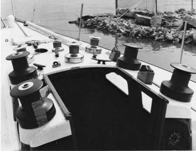
Figure 14-16 Bonded hardware on the deck and cabin top of IOR ½-ton racer Hot Flash . Several of the fittings have pads that were cast in place.
