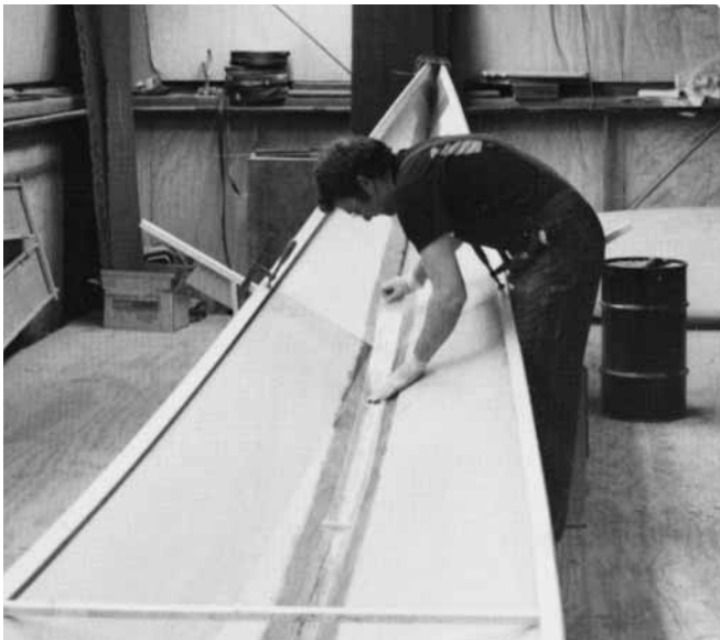
Figure 25-10 Applying glass tape over a keel fillet on a 30' (9.1m) hull.
