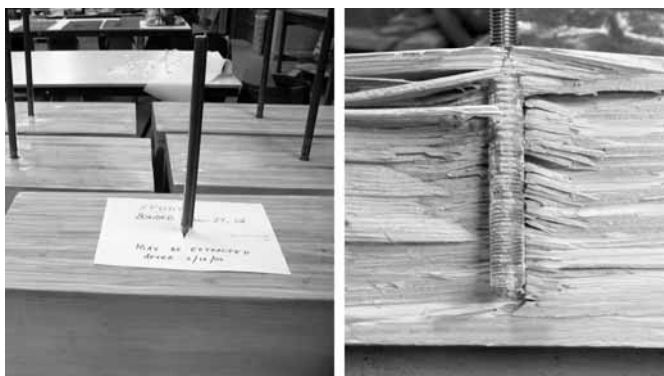
Figure 14-3 The \frac{3}{4} " test samples before testing (left) and a cutaway of the damage after testing (right). Threaded rods were imbedded parallel to the glue joints.
