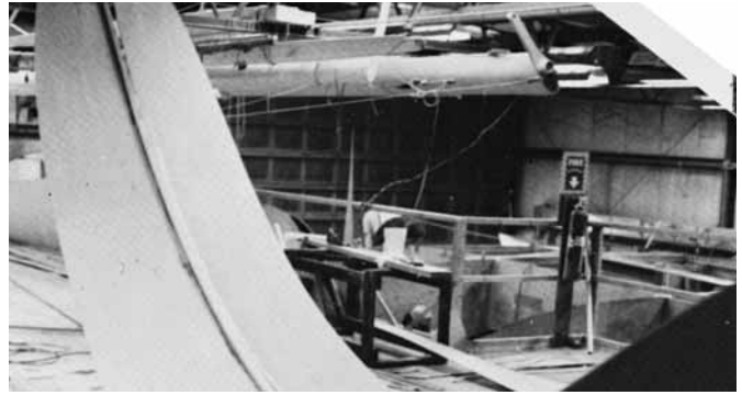
Figure 25-3 Plywood panels and sheer clamps laminated to a large curve to help develop fullness in the upper sheer area of the completed hull.
