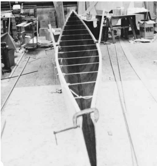
Figure 25-14 Folding up a 30' trimaran hull with drawstrings. Note that the sheer clamps have been beveled at the stern so they can be clamped together when the hull is folded up.
