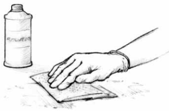
Figure A-6 Clean the surface. Use an appropriate solvent as necessary to remove contaminants.
