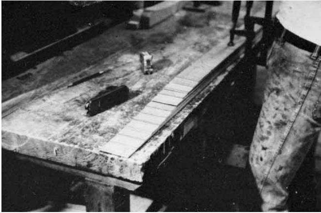
Figure 12-11 Planing narrow plywood strips with a block plane.
