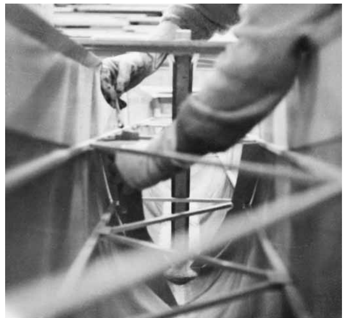
Figure 25-17 Struts and bracing for sub-level stringers in a Tornado catamaran hull. Note the small plywood gussets holding the struts to the stringers. Small plywood half frames are being installed against the hull skin. These frames will be filleted to the skin. The centerboard case is the vertical structure in the middle of the hull.
