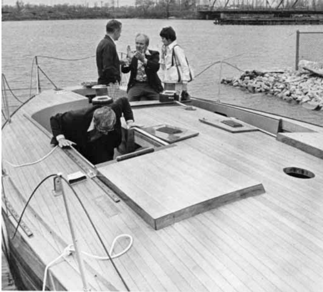
Figure 27-35 Teak planking on Golden Dazy laid parallel to the centerline. Installation was simplified because strips did not have to bend to the arc of the sheer line.
