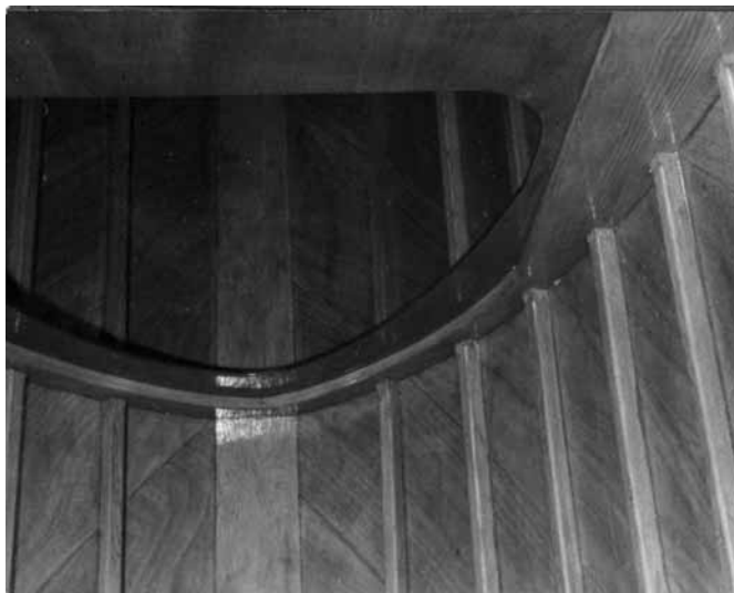
Figure 26-28 A clean, well finished interior built with WEST SYSTEM epoxy.
