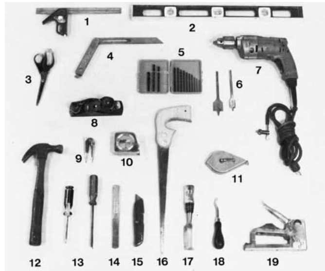
Figure 8-1 Minimal small tool inventory: (1) combination square; (2) 24-inch level; (3) scissors; (4) sliding bevel or bevel square; (5) basic drill bit assortment; (6) spade drill bits as needed; (7) electric drill motor; (8) block plane; (9) compass; (10) 25-foot tape measure; (11) chalk line; (12) hammer; (13) screwdrivers; (14) rasp; (15) utility knife; (16) keyhole saw; (17) chisel; (18) staple removing tool; (19) staple gun.
