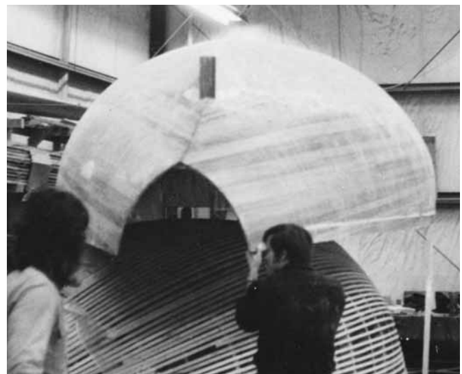
Figure 21-24 A molded hull being lifted from a ribband mold. The protective plastic sheet can be seen on the stern of the mold.
