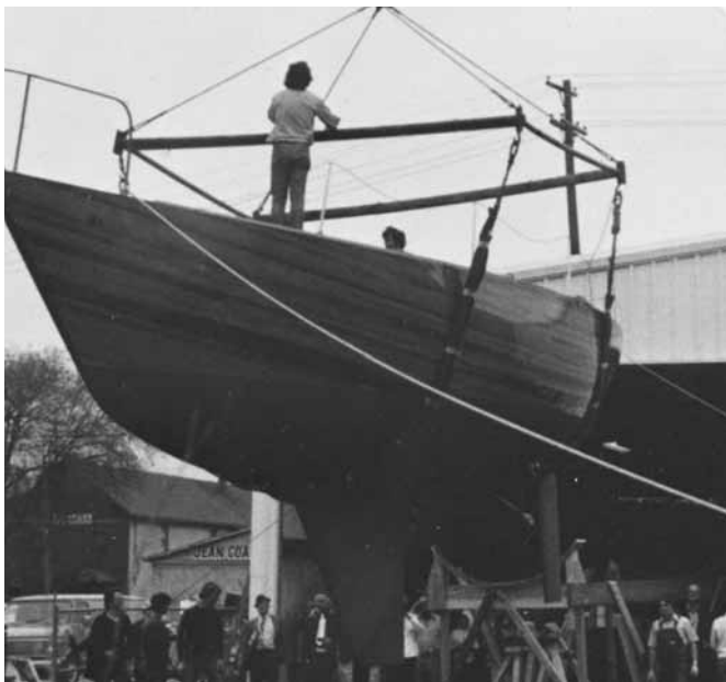
Figure 23-11 Launching the 42' yacht. The natural finish highlights the final layer of veneer laid fore and aft.
