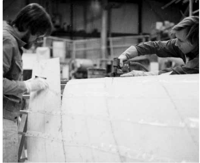
Figure 21-15 Applying an adhesive epoxy mixture to the edge of a cedar plank.
