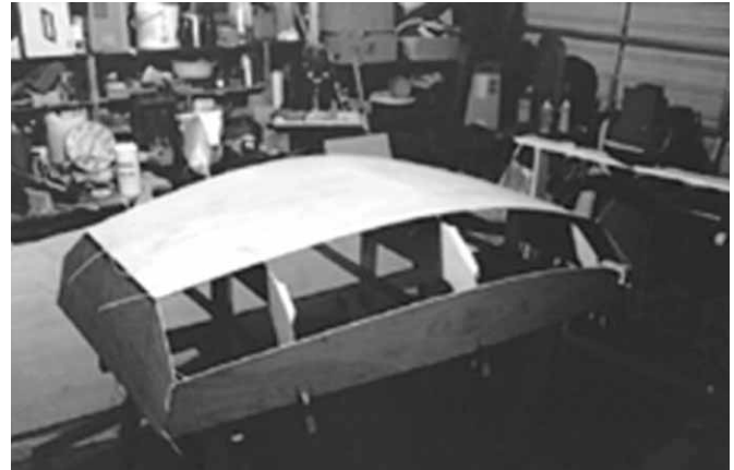
Figure 24-11 A stitch-and-glue pram under construction. Frames will hold the shape until stitching is complete. A brace across the gunwales will hold the shape while the hull is inverted and the interior joints are filleted and taped.
