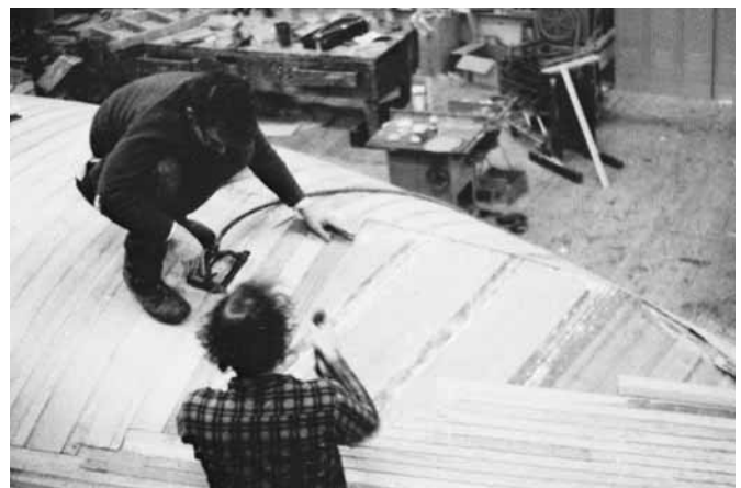
Figure 21-21 Applying the final layer of veneer on IOR 2-ton Golden Daisy . Topsides of this layer were laid fore and aft, and bottom veneers laid athwartship and butted as in the photo. Note that the layer of veneer below the final layer is of much wider veneers.
