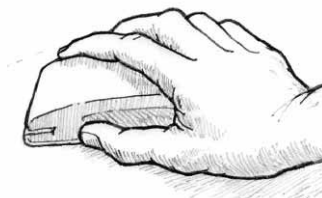
Figure A-8 Sand non-porous surfaces. Provide a texture for the epoxy to key into.
