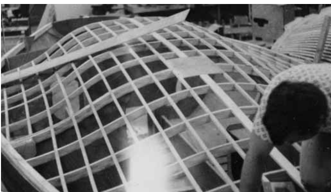
Figure 27-11 Laminated frames and 1" × 3/4" (25mm × 18mm) stringers used as framing for a blister-type deck on a 1/2 ton racer. Note the plywood mast partner for a keel-stepped spar.
