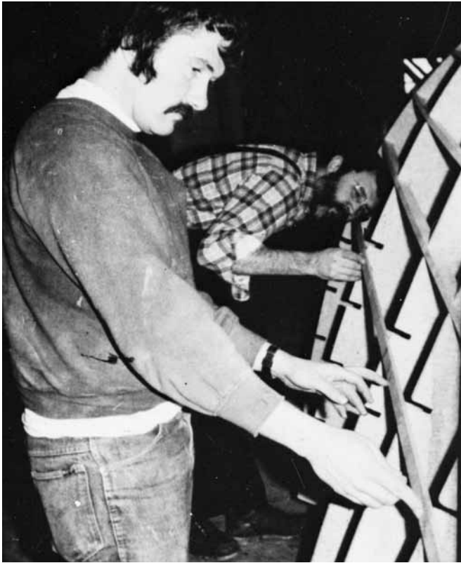
Figure 22-7 Fairing the molds on a stringer-frame set-up.
