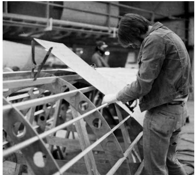
Figure 21-9 Fitting the first layer of cedar veneer for a laminated hull. The plank is secured in the middle, then the ends are adjusted and fitted to an adjoining plank.
