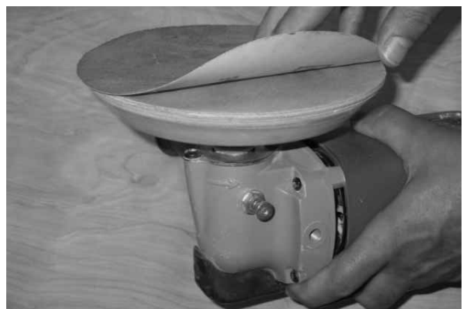
Figure 8-6 A foam disc pad used with the 7" electric orbital polisher. We bond a piece of ¼" birch plywood (or plastic laminate) onto the face of the disc. The plywood is flexible enough to follow major contours, yet is effective for sanding and fairing uneven surfaces with varying densities, such as cured epoxy with various fillers.
