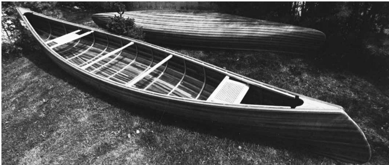
Figure 23-12 Two stripper canoes built by Herschel Payne. Western red cedar and WEST SYSTEM epoxy were used for both boats. The 15' (4.5m) model weighs 32 lb (12.8kg) and the 18' (5.5m) model weighs 48 lb (21.6kg) .
