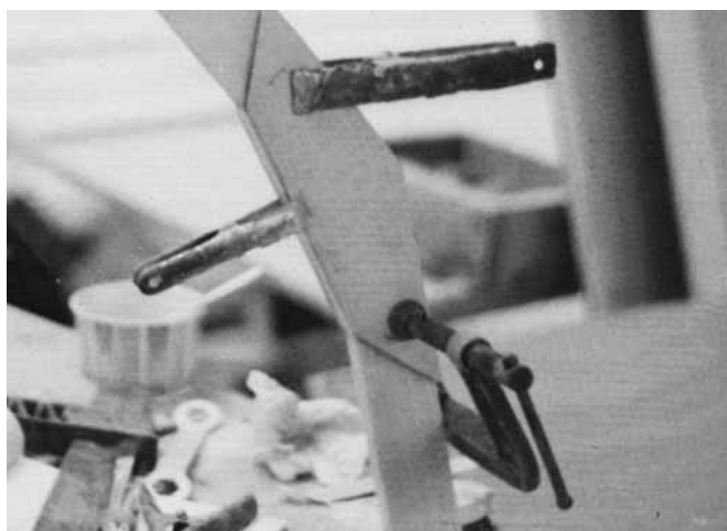
Figure 17-6 Bonding gussets to permanent frames.
