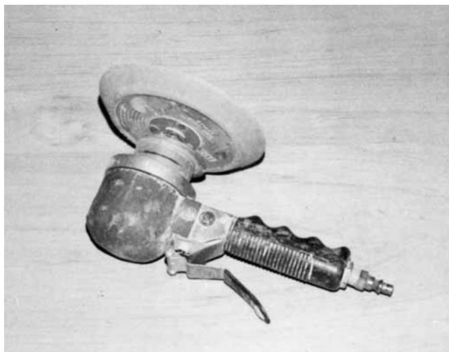
Figure 8-8 A 7" electric orbital polisher is used with a foam disc pad for sanding.
