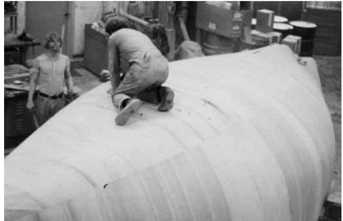
Figure 21-23 This hull is being finish sanded in preparation for epoxy coatings. Note the veneer seam along the bilge. Topsides on this hull were choice veneers carried from the sheer to just below the waterline.
