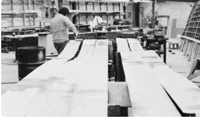
Figure 22-13 Coating 40' × 1' (1200mm × 2400mm) panels of planking stock. Scarfing together long lengths of planking stock like these cuts down on scrap rate.
