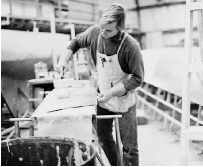
Figure 21-16 Rolling an epoxy mixture, slightly thickened with low-density filler, onto cedar veneer with a foam roller.
