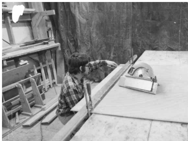
Figure 12-6 Setting up a straightedge for the Scarffer attachment.
