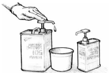
Figure A-2 Dispense the proper proportions of resin and hardener. With Mini Pumps—pump one full stroke of resin for every one full stroke of hardener.
