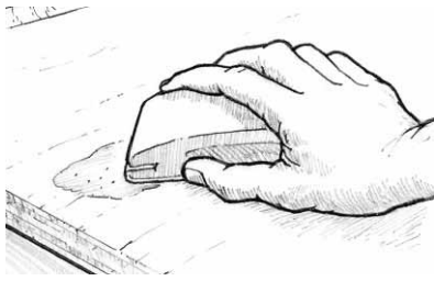
Figure A-23 Sand cured fairing compound to the desired contour.
