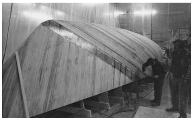
Figure 23-9 Laminating a second layer of veneer onto a strip planked hull.
