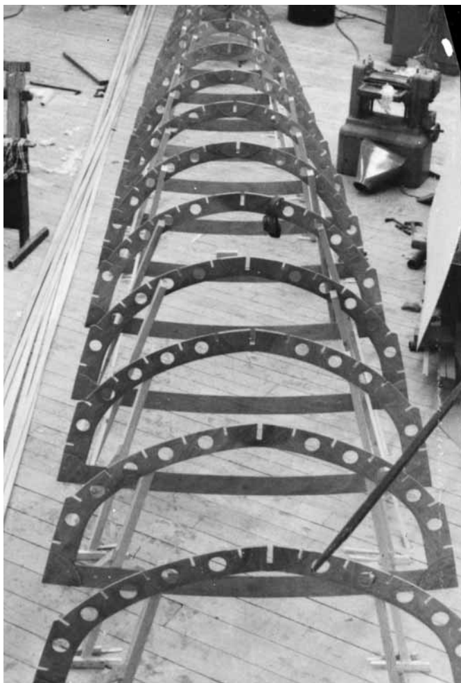
Figure 22-2 Frames set up for the proa Slingshot . In this case, stringers for the bottom were marked off parallel from the chine and run out toward the keel. The single topside stringer was centered between the sheer and the chine.
