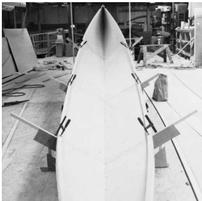
Figure 25-7 Panels for a trimaran outrigger hull showing temporary frame supports.
