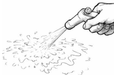
Figure A-33 Rinse the surface with fresh water after sanding.
