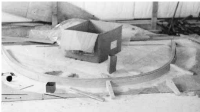
Figure 11-5 Cleats are screwed to a baseboard to force laminates into the shape required. Clamps in the pile in the upper right will be used during the dry run and the final lamination.
