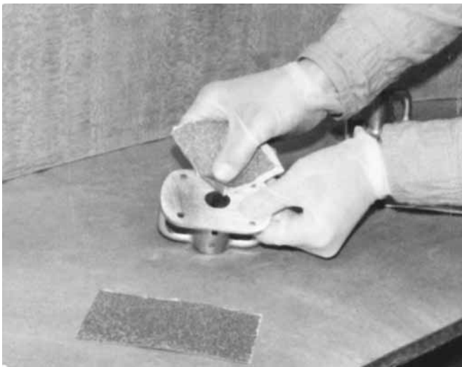
Figure 14-12 Sand the bonding surface of steel and bronze fittings with coarse sandpaper.
