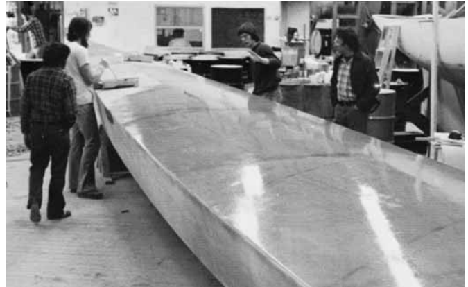
Figure 15-3 Building up epoxy coating on the deck of the proa Slingshot . Note that the topsides and bottom have been coated with gray pigmented epoxy.
