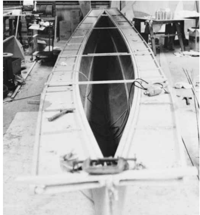
Figure 25-16 A folded 30' hull with sub-level stringers laminated on the inside.
