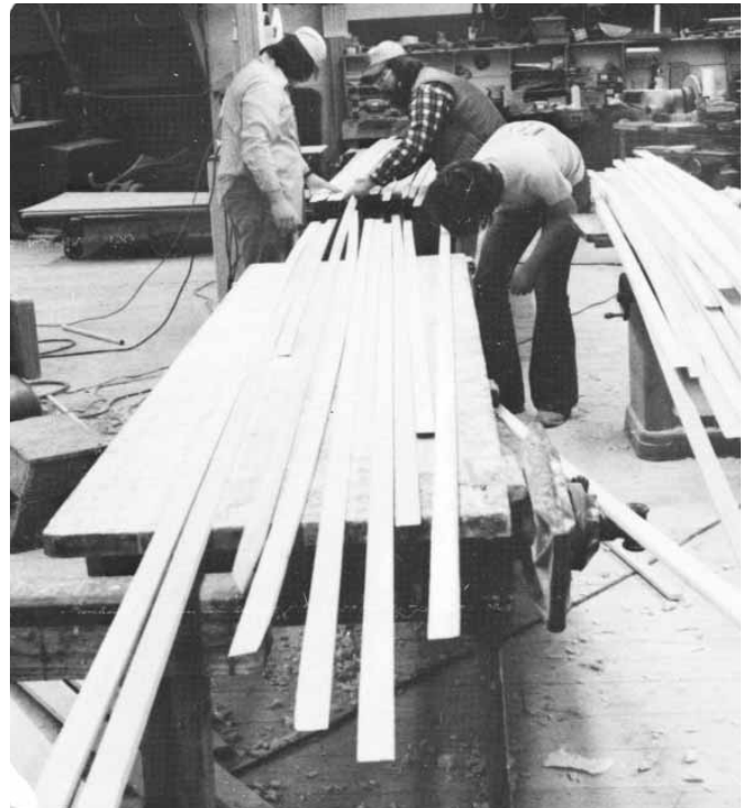
Figure 12-4 Stringers being prepared for bonding and clamping. Scarf bevels have been cut on both ends. This set-up places scarfs close to each other to minimize the number of clamps needed.
