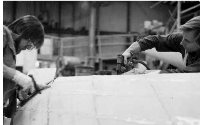
Figure 21-7 Stapling veneer plank to a hull's stringers. Note the use of plastic strips under the staple heads to ease removal.
