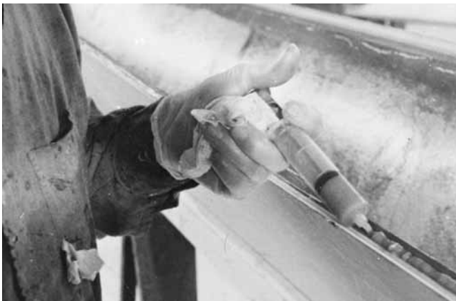
Figure 11-19 A disposable syringe being used to apply a bead of thickened epoxy.
