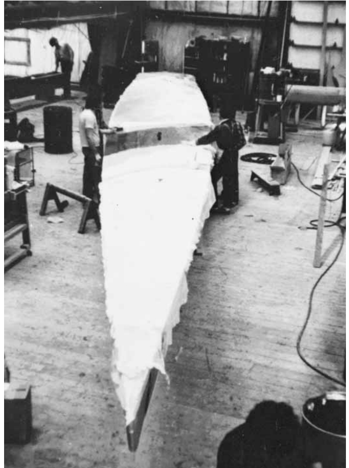
Figure 13-1 Applying fiberglass to the deck of the 60' (18.2m) proa Slingshot using the dry method. Applicators have wet out the glass cloth around the daggerboard slot and are working toward the bow and stern.
