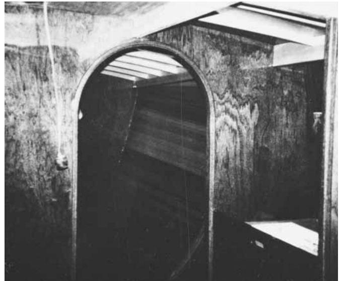
Figure 26-13 A bulkhead showing laminated hardwood trim on the walk-through.
