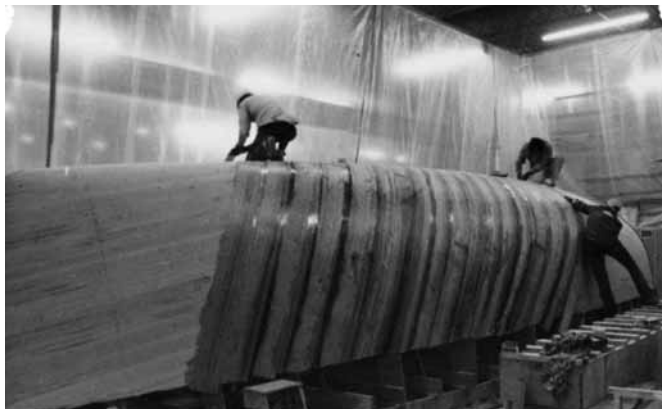
Figure 23-8 Laminating the first layer of veneer over faired planking. Note the planking bench to the right.
