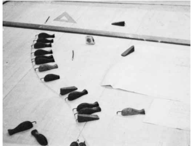
Figure 16-7 Lofting weights and a flexible plastic batten being used to fair after sections on an IOR racer.
