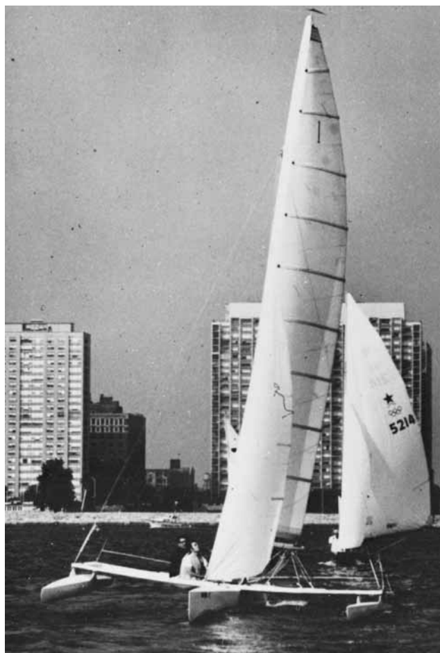
Figure 25-1 Victor T , a lightweight, 25' (7.6m) C-class trimaran, was built using compounded plywood technique.
