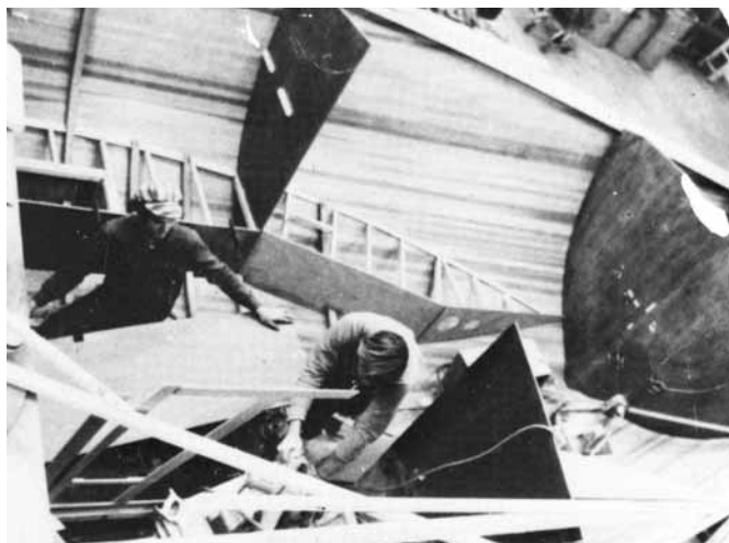
Figure 26-1 Six bunks, a galley, and shelves bonded to the interior of this hull skin contributed to a noticeably stiffer structure.
