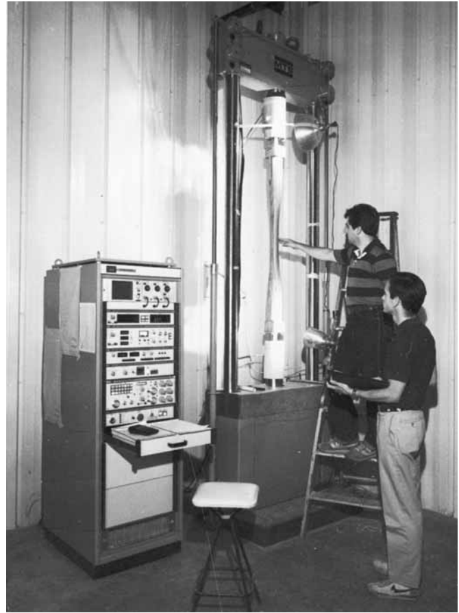
Figure 3-2 This Douglas fir laminate augmented with carbon fiber failed in compression at about 20,000 psi.
