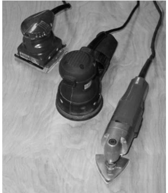
Figure 8-9 A selection of electric sanders: 4" finishing sander, random orbital sander, and detail sander.
