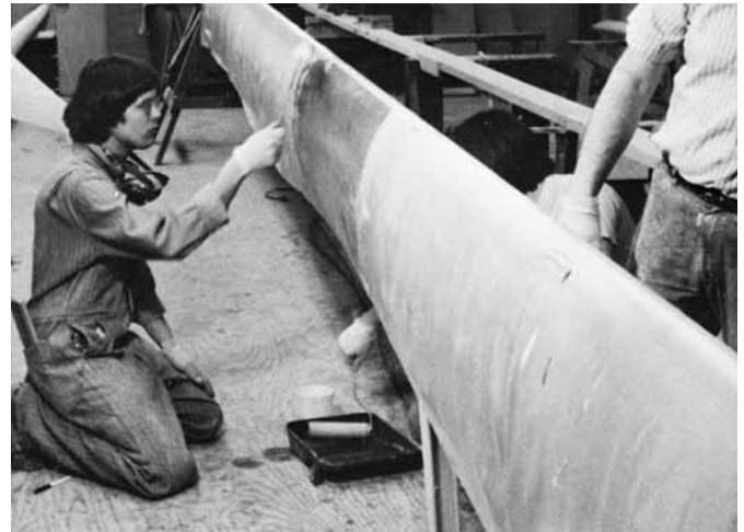
Figure 13-4 Wetting out the fiberglass cloth on a wing mast for the 60' proa Slingshot . In this application, 4 oz cloth was draped over the spar and wet out with rollers.
