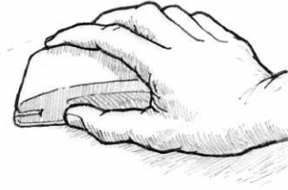
Figure A-32 Sand the surface to a smooth finish.
