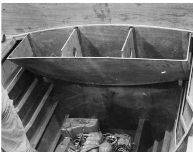
Figure 26-24 A diesel fuel tank on Rogue Wave . The cockpit sole forms the top.
