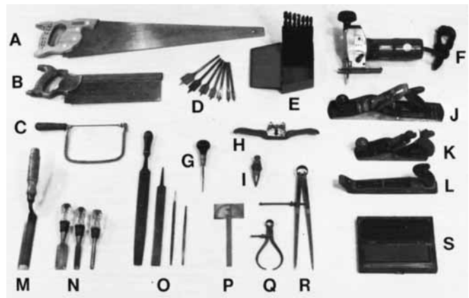
Figure 8-2 Broader small tool inventory: (A) crosscut saw; (B) back saw; (C) coping saw; (D) large set spade bits; (E) large drill bit assortment; (F) electric saber saw; (G) awl; (H) spokeshave; (I) plumb bob; (J) jack plane; (K) bench or smoothing plane; (L) Surform™ tool; (M) offset chisel; (N) chisel assortment; (O) file and rasp assortment; (P) protractor; (Q) calipers; (R) dividers; (S) whetstone.
