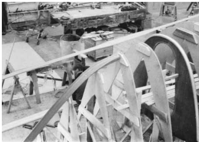
Figure 19-3 Set-up for the 42' (12.8m) Golden Dazy . The keel can be seen on sawhorses beyond the molds. The slight rocker in this hull allowed the use of a solid keel.
