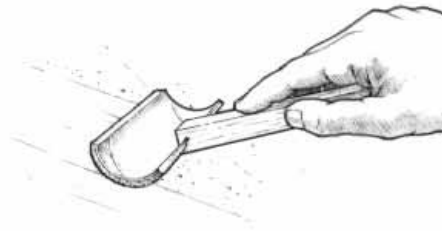
Figure A-31 Tip off the coating by dragging a foam roller brush lightly over the fresh epoxy.
