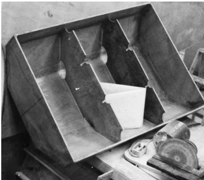
Figure 26-23 A 40-gallon (150 liter) tank for Rogue Wave , constructed using fillets and fiberglass tape on all inside joints. The top of this tank forms a part of the cabin sole and the tank is removable. Baffles are scalloped on the upper edge so each compartment will vent. Notches at the bottom of the scallops are for \frac{3}{8} " (9mm) thick longitudinal plywood frames to support the top.
