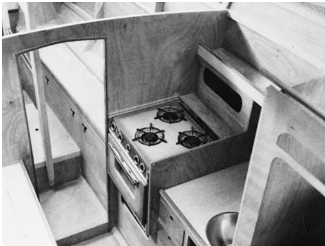
Figure 26-16 A galley in a 30' (9.1m) trimaran with a bulkhead forward and a hanging locker at lower right.
