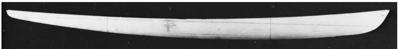
Figure 25-34 A model of the outriggers shown in Figure 25-27. This model has been marked with waterlines and section lines.
