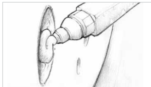
Figure 12-3 Wet out the cleaned blister cavities with unthickened epoxy.
