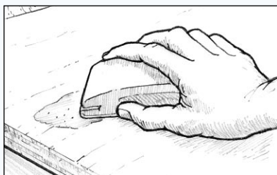
Figure 23 Sand cured fairing compound to desired contour.
