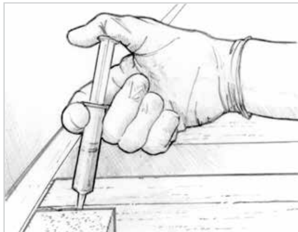
Figure 4-8 Inject epoxy as far as possible into the joint.
