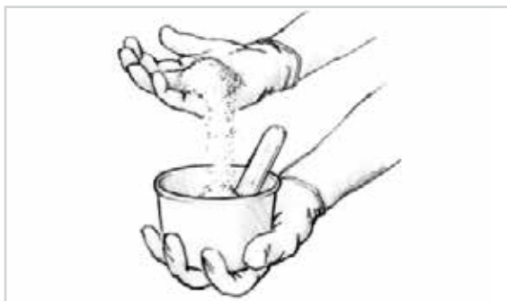
Figure 8-7 Blend in small handfuls or scoops of the appropriate filler until the desired consistency is reached.
