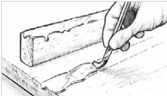
Figure 8-8 Wet out bonding surfaces with unthickened epoxy for maximum penetration and greater adhesion.
