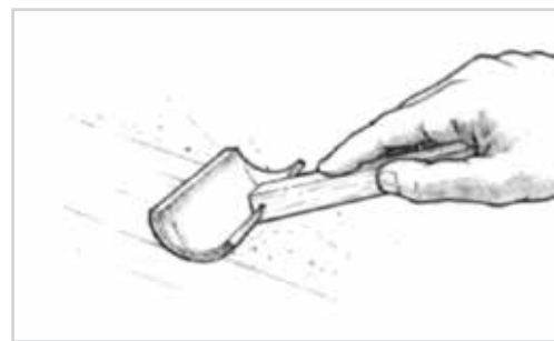
Figure 7-4 Tip off the coating by dragging a foam roller brush lightly over the fresh epoxy.
