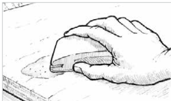
Figure 8-16 Sand the fairing material to blend with the surrounding contour.
