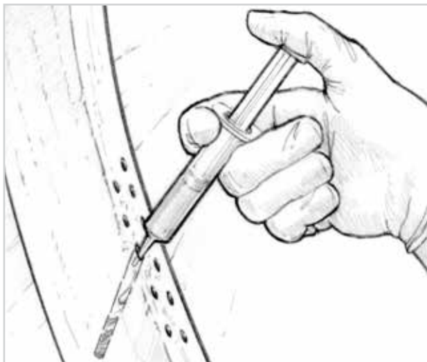
Figure 3-4 Inject resin/hardener mixture into holes until the damaged wood absorbs all it can.
