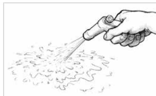
Figure 7-6 Rinse water should sheet without beading, indicating an uncontaminated surface.
