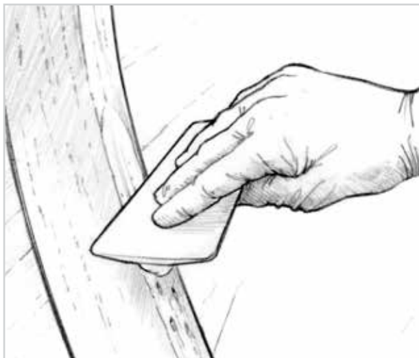
Figure 3-5 Fill the remaining voids with fairing compound.
