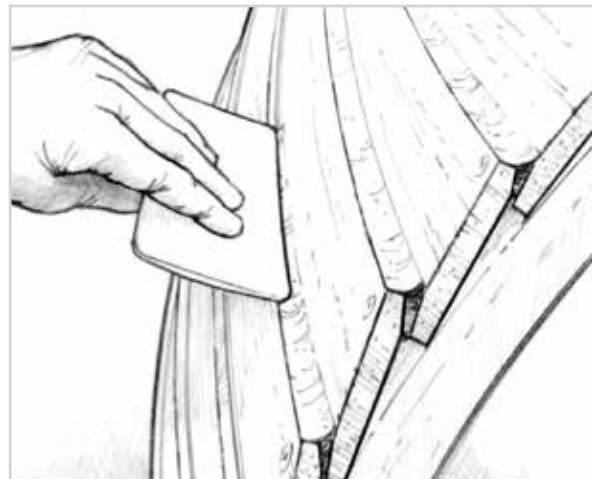
Figure 5-9 Fill the wet-out seam with thickened epoxy.
