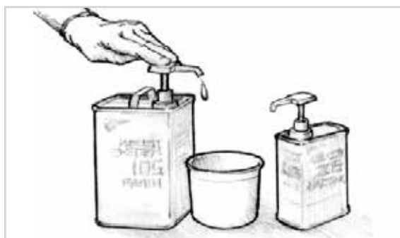
Figure 8-4 Dispense the proper proportions of resin and hardener.
