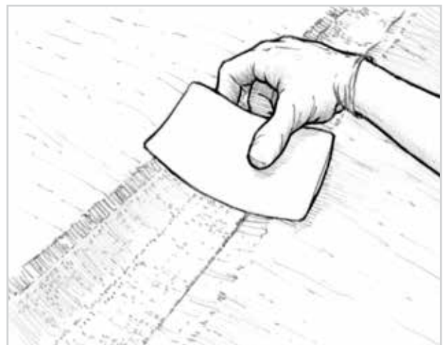
Figure 5-11 Apply fiberglass tape over the prepared joint.
